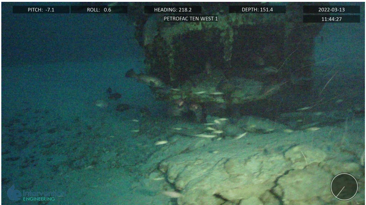
Figure 8 Ten West 1 example broken grout on seabed
