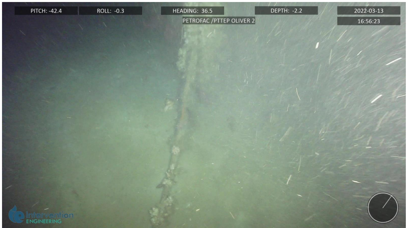
Figure 15 Oliver 2 Guide wire remnant in contact with seabed
